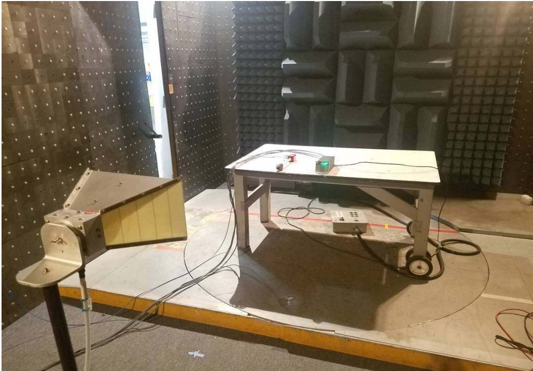
Test Configuration Photograph #2 (Radiated Immunity, EN 61000-4-3)
