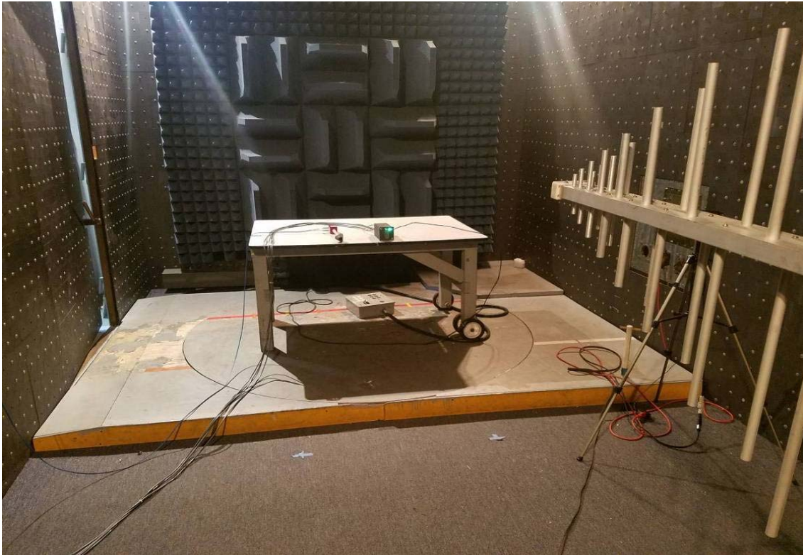
Test Configuration Photograph #1 (Radiated Immunity, EN 61000-4-3)
