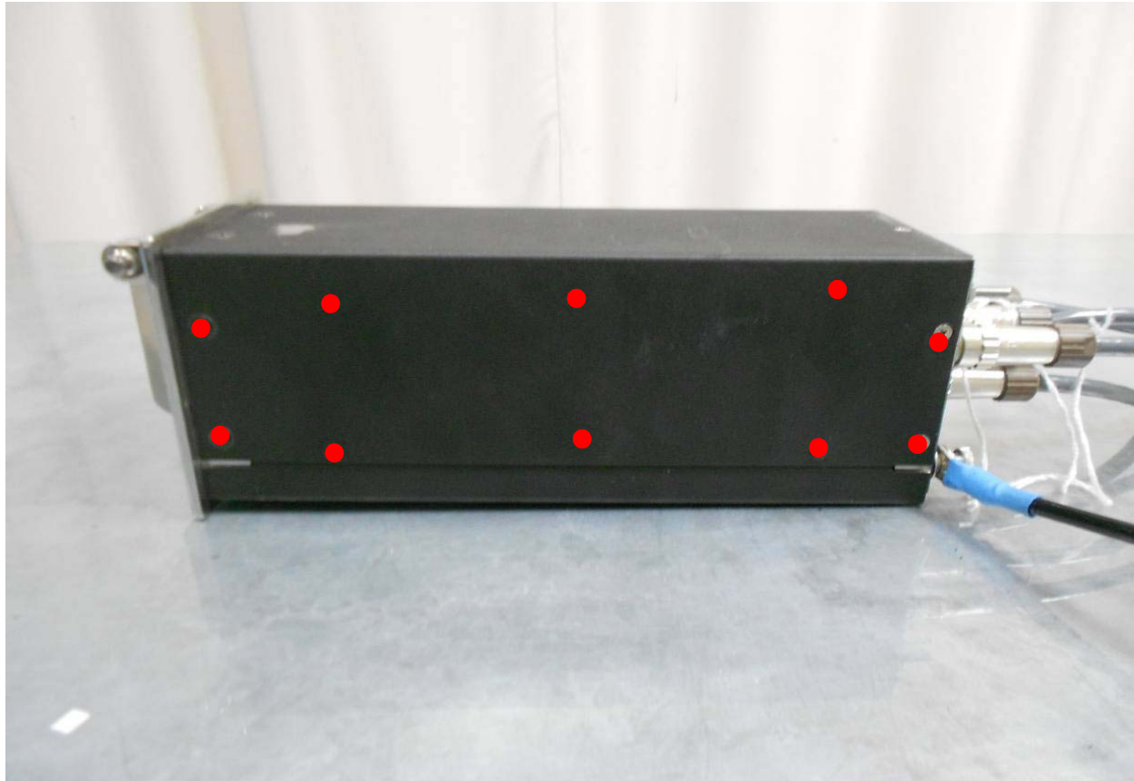
Detailed Photo(s) of ESD Test Locations
