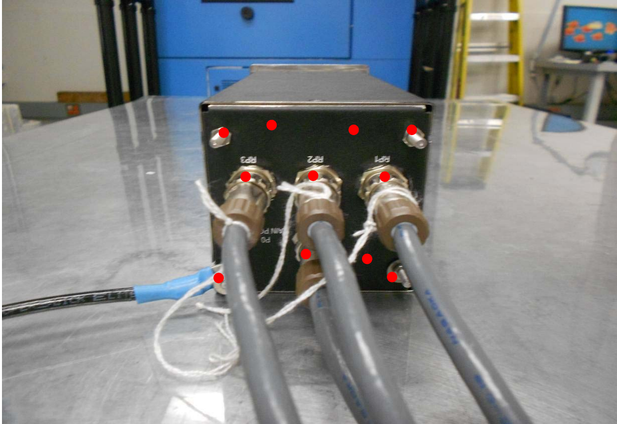
Detailed Photo(s) of ESD Test Locations
