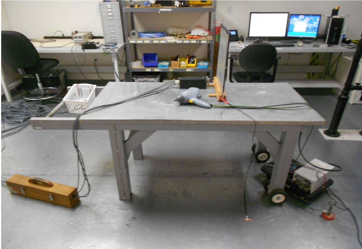
Test Configuration Photograph [General View of Test Setup - Alternate View] (Electrostatic Discharge, EN 61000-4-2)
